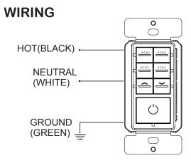
\* Switched Hot to Load is not required. Switching is done at the power pack or in-fixture load controller.
